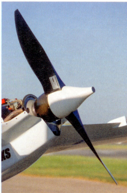
THIS FIXED-PITCH , carbon-fiber propeller with a massive twist of more than 100 inches is optimized for the Determinator .
